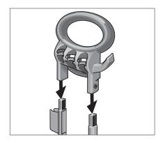
**Step 3** Before pressing down handle onto top of adapter brackets, the hose/cord caddy and trigger gun holder must be on opposite sides.
